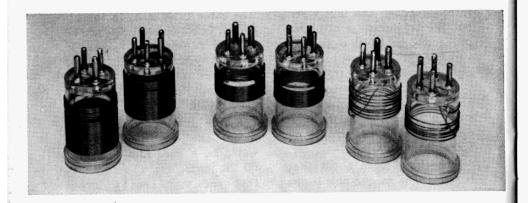
plug in like a radio tube to cover different broadcast bands. They are easily wound on ready-made plastic forms available at parts suppliers. Use the specifications on page 35, and the winding guide below. Be careful in soldering the wires in the coil-form pins. The polystyrene forms will soften if heat is applied to the pins for a short period.
